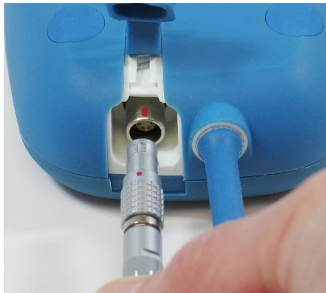
Figure 83: Alignment of the Bootstrap Loader Cable and Guardio/Vesta Charger Connectors
